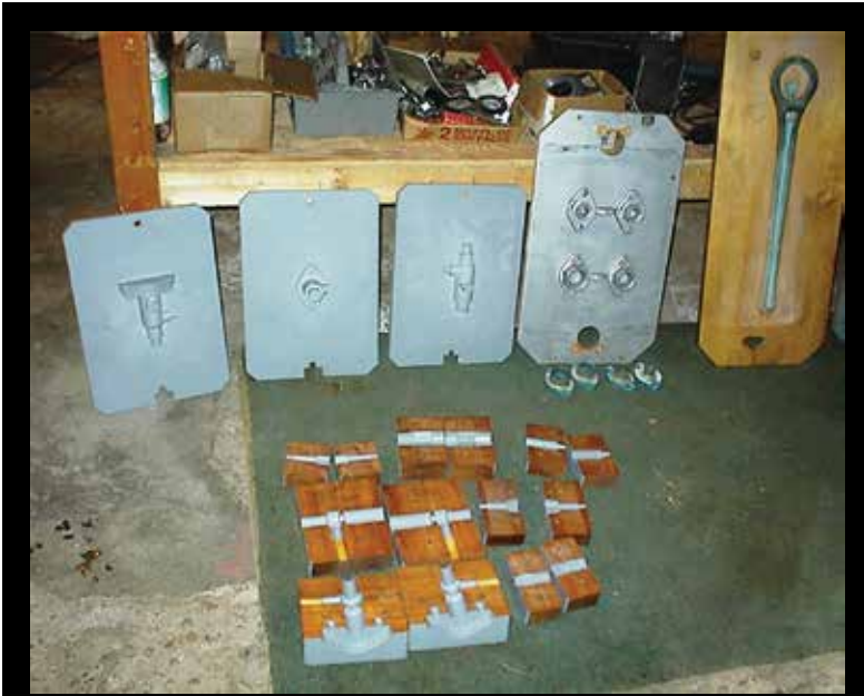
Figure 23: The flange and valve patterns that produced the prototypes (figure 21).
